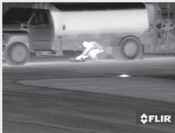
Thermal cameras detect humans, vehicles, and objects in complete darkness and other low-visibility conditions.
